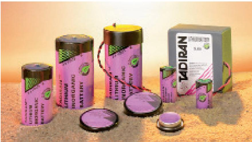
» A good long-term power solution for a remote wireless device is a bobbin-type lithium thionyl chloride ( $\text{LiSOCL}_2$ ) battery, which features the highest capacity and highest energy density of any lithium chemistry, along with a very low annual self-discharge rate, the widest possible operating temperature range, and a hermetic glass-to-metal seal to help prevent battery leakage.
