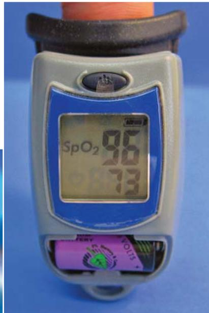
First utilized in pacemakers during the 1960s, primary lithium batteries now power all types of medical devices, including this wireless blood oxygen meter. (Above)
