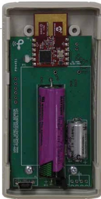
However, for a different application, the WSN-1101 wall-mounted sensor, Powercast chose to power the device with a hybrid LiSOCL<sub>2</sub> battery instead of using energy harvesting.
