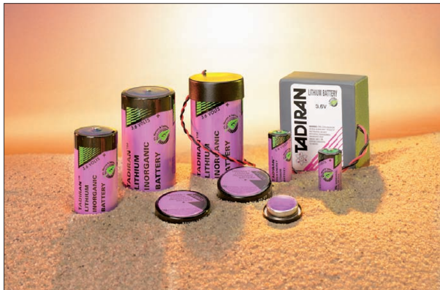
Bobbin-type lithium thionyl chloride (LiSOCl 2 ) batteries are preferred for remote wireless applications because they deliver high energy density with up to 40+ years of service life and the widest possible temperature range, making them ideal for use in extreme environmental conditions.
