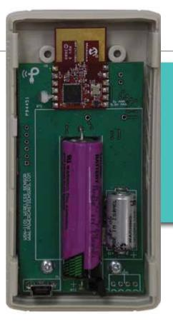
However, for a different application, the WSN-1101 wall-mounted sensor, Powercast chose to power the device with a hybrid LiSOCL<sub>2</sub> battery instead of using energy harvesting.
