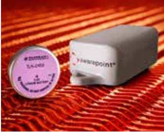
Awarepoint medical asset tracking RFID tags contain bobbin-type LiSOCl 2 batteries that can withstand high temp. autoclave sterilization without having to remove the battery, saving labor and providing a continuous data stream.
