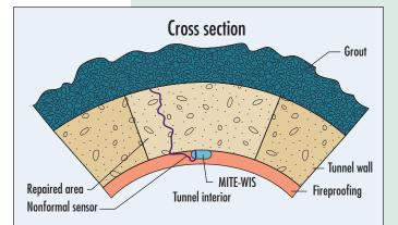
A wireless MITE-WIS unit embedded in a concrete repair patch enables fireproofing material to maintain its integrity by eliminating the need for large cables to pass through tunnel-wall concrete, which would otherwise create weak points for heat infiltration.
