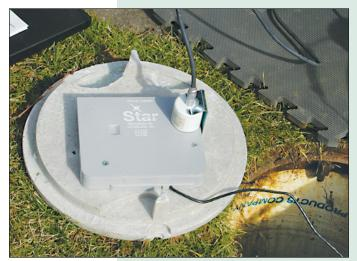
Hexagram STAR meter-transmitter units contain lithium cells that are still operating after 20 years in the field.
