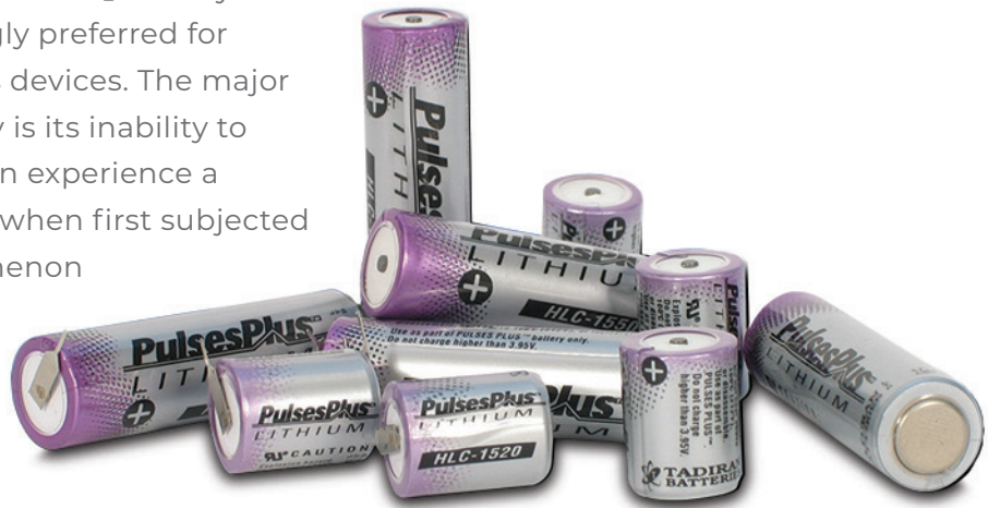
Figure 3. PulsesPlus cells combine a standard bobbin-type \text{LiSOCl}_2 battery with a hybrid layer capacitor (HLC) to deliver high pulses to power two-way wireless communications.
