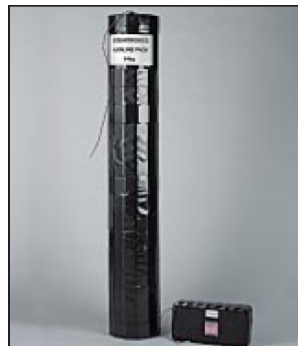
Same operating life with smaller size for use in GPS/ice buoys. Oceantronics' original battery pack (left) used 380 alkaline D cells (54 k). The new battery pack (right) uses 32 lithium thionyl chloride D cells and four hybrid layered capacitors (3.2 kg).
