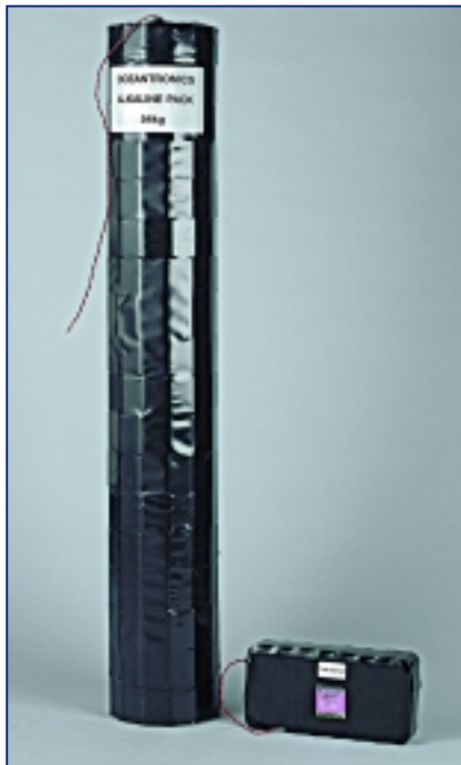
Same operating life with smaller size for use in GPS/ice buoys. Oceantronics' original battery pack (left) used 380 alkaline D cells (54 kg). The new battery pack (right) uses 32 lithium thionyl chloride D cells and four hybrid layered capacitors (3.2 kg).
