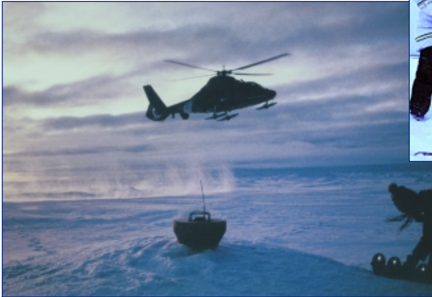
Oceantronic's GPS/ice buoy being retrieved by helicopter to the Arctic for use in experiments measuring wind, temperature sunlight and ice thickness near the North Pole. (Courtesy Sigrid Salo NOAA/PMEL.)
