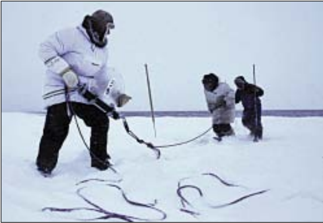
Nortek's Aquadopp GPS current meter being installed by Canadian Wildlife Service as part of a field study in Hudson Bay. The Aquadopp is used to study the effects of tidal currents on eider ducks in areas near the open ocean in seas otherwise covered with ice. (Courtesy of Grant Gilchrist, Canadian Wildlife Service.)
