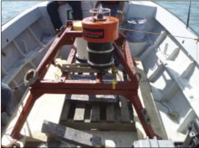
Modular bottom frame with Teledyne RDI ADCP and Benthos Pop-Up buoy.
