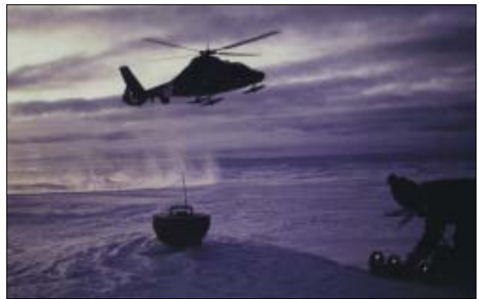
Oceantronics’ GPS/ice buoy being retrieved by helicopter to the Arctic for use in experiments measuring wind, temperature sunlight and ice thickness near the North Pole. (Courtesy Sigrid Salo NOAA/PMEL.)
