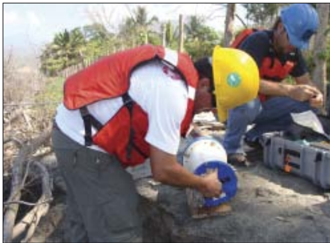
Golder team member servicing a Teledyne RDI ADCP on a beach in Colombia.
