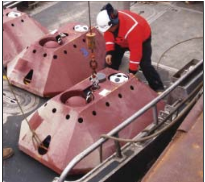
Nortek AWAC acoustic Doppler current profiler, photo taken in Beaufort Sea, AK, 2008, courtesy of Dr. Bruce Magnell, Woods Hole Group, Inc.
