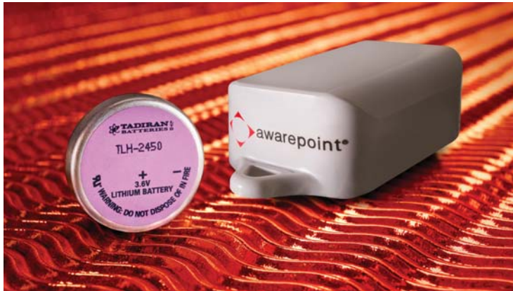
Awarepoint developed an RFID asset tracking tag for medical applications that uses lithium thionyl chloride batteries capable of withstanding the high temperatures associated with autoclave and chemical sterilization cycles.
