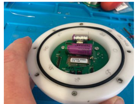
↖ Cryoegg monitors temperature, pressure, and electrical connectivity by transmitting data underwater via radio waves, powered by bobbin-type LiSOCl 2 cells. (Credit: Cardiff University)
